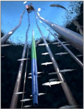
The second trip BHA comprises the Gator Perforator, which is run to a depth of 954 meters—10 meters above the MEGA PACKER casing plug.
