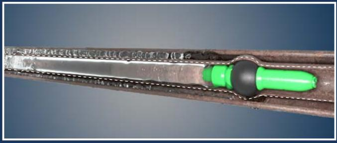
Fluid Cleans Mud down to B-Annulus Diversion at MPX Casing Expansion
