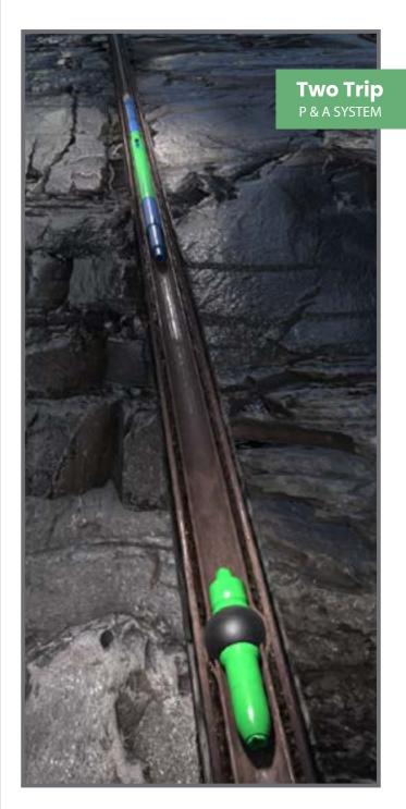
Once at depth, the Gator Perforator is pressurized to complete a series of perforations above the MPX plug and higher up in the welbore. Three perforations spaced 1 meter apart, at the lower and upper interval were completed to prepare the well for circulation and cementing.
