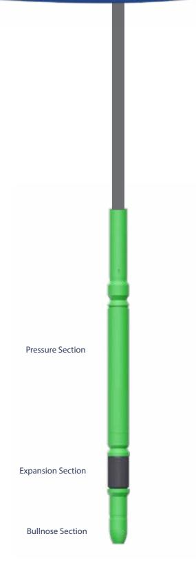
NOTE: Casing Expansion with the 838-MPX begins at approximately 50 psi for the 9-5/8, 47 lb/ft, L80 casing where the packer will lock onto the casing.
