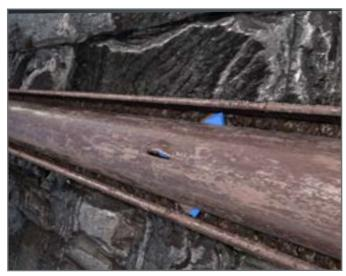
Perforations feature a large open flow area and extend into the outer annulus, enhancing casing centralization and facilitating effective annular cleanup and cement displacement. Through hydromechanical means, four radial perforations are achieved, spaced 90 degrees apart, guaranteeing excellent radial coverage with no ID burrs or internal damage to the casing.
